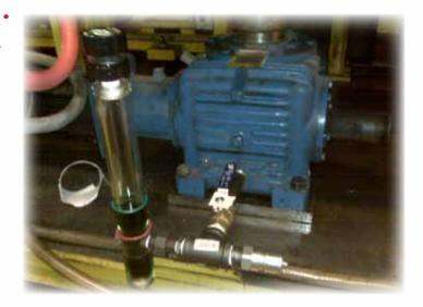
the gearbox drain ports to make oil drains easier. He suggested that the operator simply attach the hose from an existing filter cart to the AMS Quick Connect whenever the oil needed to be drained, then use the cart as a convenient transfer unit to get rid of the used oil.
